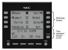
32 (8 keys x 4 pages) additional programmable keys are provided. They can be programmed as Flexible Line/Programmable feature key by Telephony Server Administrator. For the SL2100, the programmable keys can be set by WebPro/ PCPro/Tel Pro and user can also set them.
