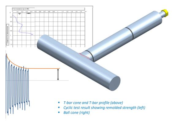
Full flow penetrometers are used to accurately determine strength characteristics of soft and very soft soils, sediments or mine tailings. Originally designed as lab instrument, the test found its way to offshore geotechnical investigations and finally to other areas of use.
