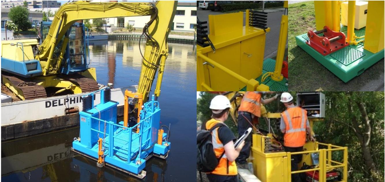
The Geomil Equipment Lizard-200 is a hitch-up Cone Penetration Testing (CPT) system to be used in combination with an excavator. It allows for conducting CPT's in near to impossible conditions, such as sites where space is limited and ground anchors cannot be used.
