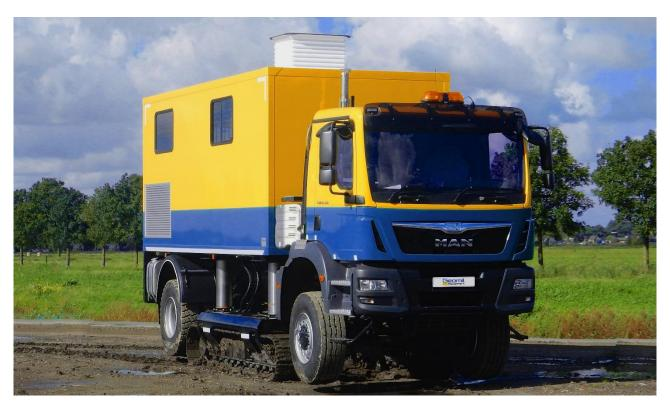
The Kodiak series is Geomil Equipment's most advanced onshore Cone Penetration Testing (CPT) solution. The unique combination of a truck with a deployable undercarriage results in the perfect mix of efficient long-distance travel and excellent terrain capabilities, even in unfavorable conditions.
