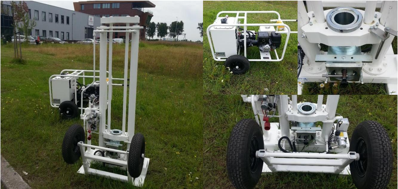
The Geomil Equipment Fox-100 stand-alone CPT system is a versatile unit designed to be used in a wide range of applications. Detachable mounting supports allow the system to be placed on any base.
