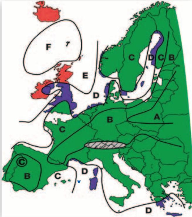
**Reference wind speeds:** Europe has therefore been divided not on national boundaries but according to a wind speed level classification (A being the lowest and F being the highest). As it can be seen, most of Europe is covered by the C category\*.
