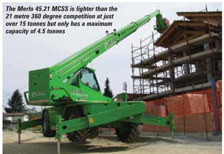
The Merlo 45.21 MCSS is lighter than the 21 metre 360 degree competition at just over 15 tonnes but only has a maximum capacity of 4.5 tonnes
