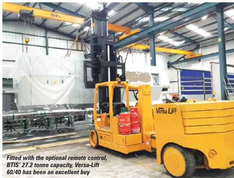
Fitted with the optional remote control, BTIS' 27.2 tonne capacity, Versa-Lift 60/40 has been an excellent buy
