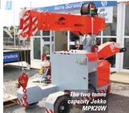
The two tonne capacity Jekko MPK20W
