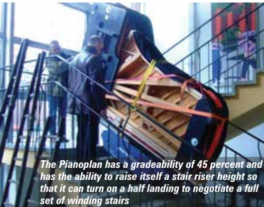
The Pianoplan has a gradeability of 45 percent and has the ability to raise itself a stair riser height so that it can turn on a half landing to negotiate a full set of winding stairs
