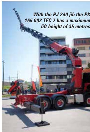
*With the PJ 240 jib the PK 165.002 TEC 7 has a maximum lift height of 35 metres*
