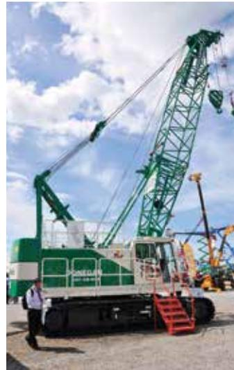
The SCX800A-3 can be rigged with up to 54.5 metres of main boom and features a nine to 18 metre jib with a maximum system length of 63.5 metres made up of a 45.5 metre boom and 18 metre jib. It can lift its maximum 80 tonnes capacity at a radius of 3.3 metres, has a minimal tail swing radius of 3.98 metres and has an overall weight of 76 tonnes.
