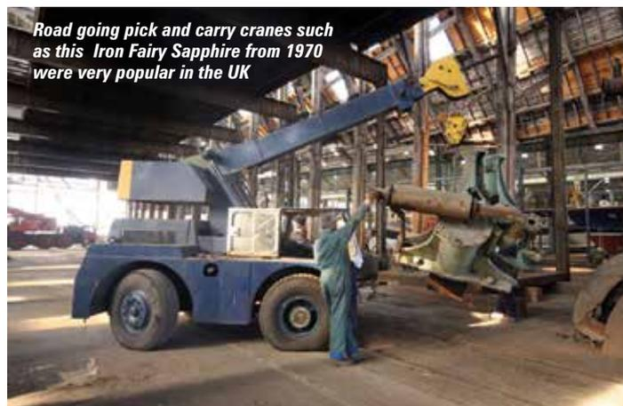
can cope with gravelled yards and they have limited boom lengths or forward reach. The American industrial Versa-Lift forklift offers an alternative to this design and has carved out a niche for itself for moving heavy machinery, being compact and having very good lift capacity but ideally needs a good surface to operate on.
