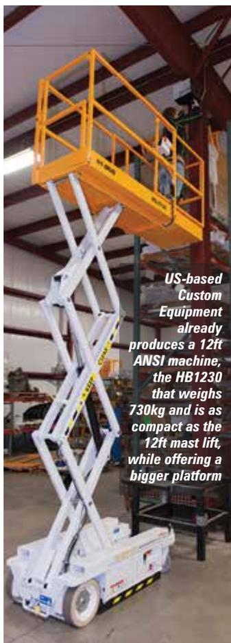
*US-based Custom Equipment already produces a 12ft ANSI machine, the HB1230 that weighs 730kg and is as compact as the 12ft mast lift, while offering a bigger platform*
