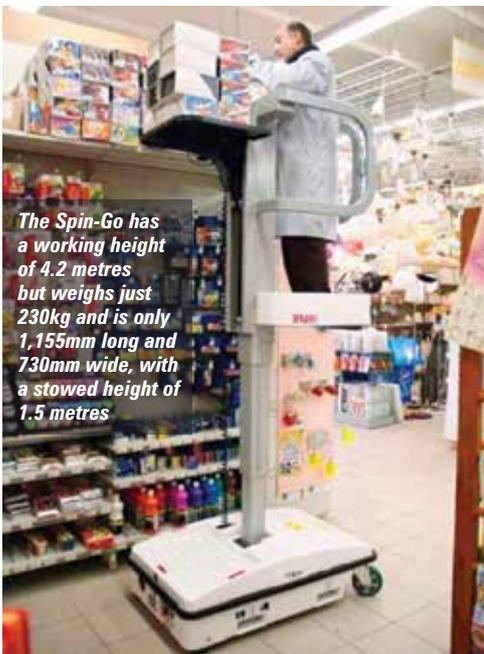
*The Spin-Go has a working height of 4.2 metres but weighs just 230kg and is only 1,155mm long and 730mm wide, with a stowed height of 1.5 metres*
