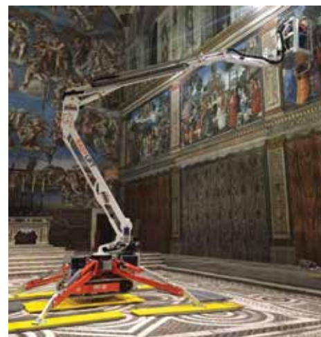
Spider in the Sistine Chapel: Earlier this year an 18 metre R180 Easy Lift R180 spider lift was used to help restore Michelangelo's frescoes in the Sistine Chapel at Vatican City, Italy. The R180 - supplied by Rome based Skylift Piattaforme Aeree - has a long riser topped by a three section telescopic boom and articulating jib for a working height of 17.6 metres, a maximum outreach of 9.6 metres with 80kg or 200kg at 7.7 metres. The retracted width of the machine is 890mm with an overall weight of 2,330kg and non-marking tracks allowing it to move through the chapel without damaging the delicate flooring.
