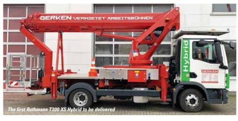
and 100kg in the platform, or 14 metres over the side. The maximum platform capacity is 250kg with the 700mm by 1.4 metre platform. A 1.6 metre wide platform with 300kg platform capacity is optional.
