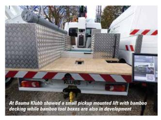
mounted lift with bamboo decking, while bamboo tool boxes are also in development. The bamboo is actually marginally lighter than the aluminium that it will replace, but most importantly is dramatically more sustainable. Klubb is sourcing locally grown bamboo, with the manufacturing carried out close to its production facility. Bamboo grows rapidly and can be harvested regularly, while requiring very few resources. It is also biodegradable.
