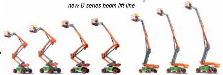
The booms feature axle-type four wheel drive, while all components are located on both sides of the chassis, simplifying routine maintenance and repair. All models can be easily transported by container with an overall width of 2.33 metres. All 21 feature jibs with 132 degrees of articulation, and an unrestricted platform capacity of 250kg.
