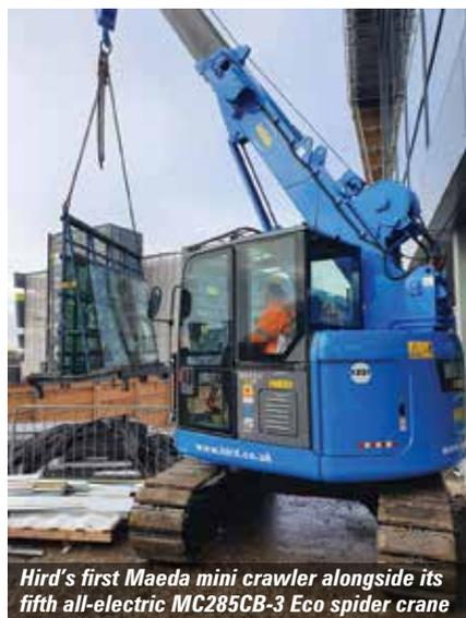
Hird's first Maeda mini crawler alongside its fifth all-electric MC285CB-3 Eco spider crane
