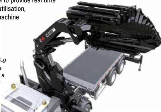
The E-8 and E-9 booms can be supplied with a six section jib
