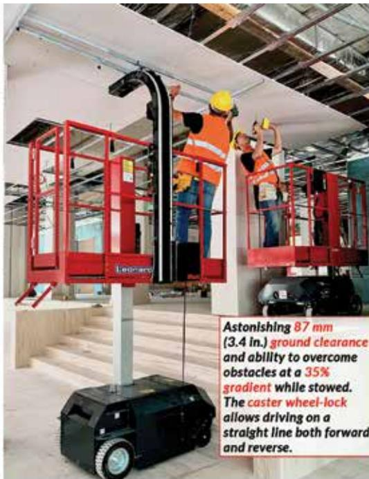
Astonishing 87 mm (3.4 in.) ground clearance and ability to overcome obstacles at a 35% gradient while stowed. The caster wheel-lock allows driving on a straight line both forward and reverse.
