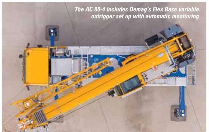
*The AC 80-4 includes Demag's Flex Base variable outrigger set up with automatic monitoring*
