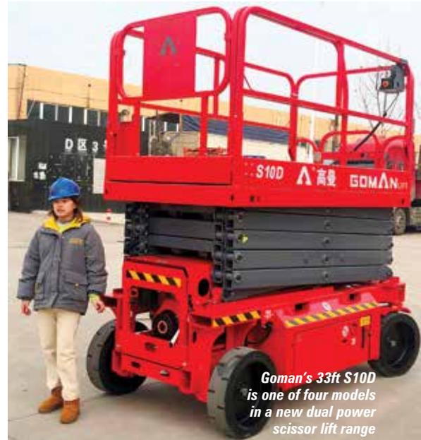
Goman's 33ft S10D is one of four models in a new dual power scissor lift range
