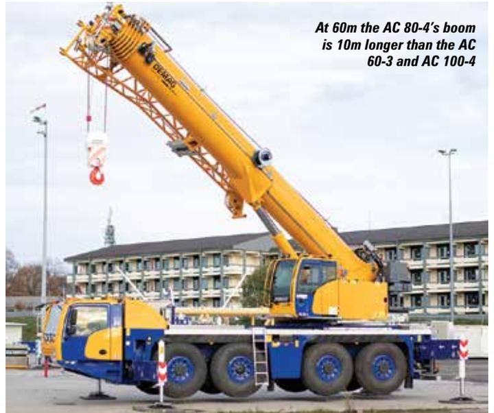
*At 60m the AC 80-4's boom is 10m longer than the AC 60-3 and AC 100-4*
