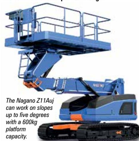
The Nagano Z11Auj can work on slopes up to five degrees with a 600kg platform capacity.
