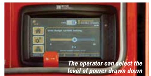
The operator can select the level of power drawn down
