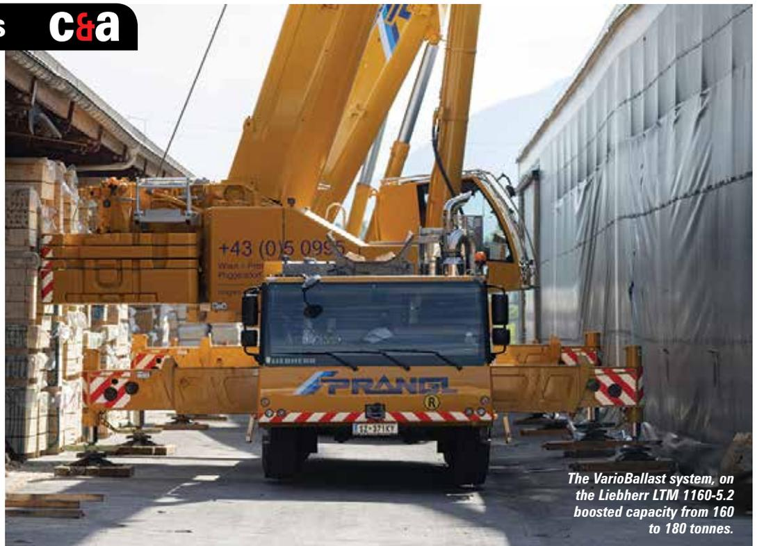
*The VarioBallast system, on the Liebherr LTM 1160-5.2 boosted capacity from 160 to 180 tonnes.*
