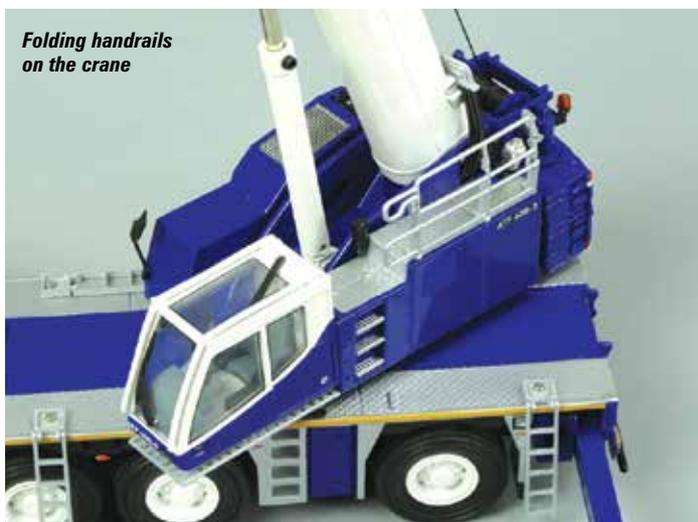
Folding handrails on the crane
