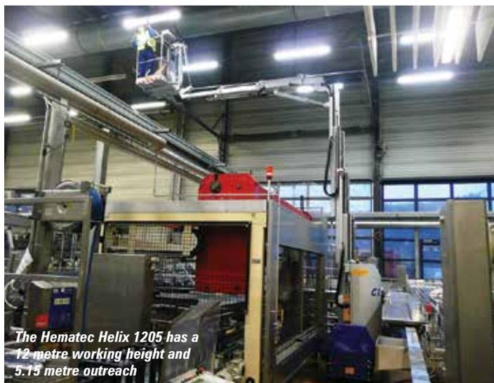
The Hematec Helix 1205 has a 12 metre working height and 5.15 metre outreach
