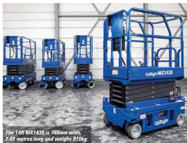
The 14ft MX1430 is 760mm wide, 1.49 metres long and weighs 810kg
