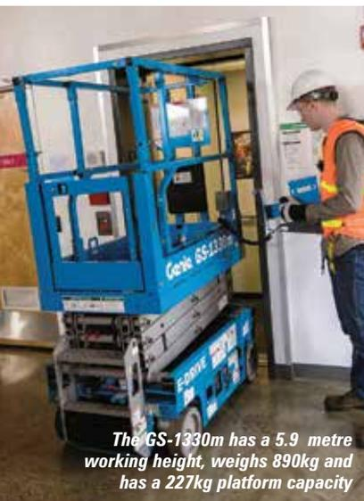
The GS-1330m has a 5.9 metre working height, weighs 890kg and has a 227kg platform capacity
