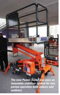
The operator can be anywhere around the machine without being restricted by the controls. By touching and holding the drive/steer controller in the track pad area, the individual can operate the machine. Haptic feedback vibration helps indicate the borders of the track pad area. Once the drive/steer controller is released, the scissor will stop, and the machine icon will move back to its home position."
