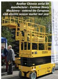
capacity of 750kg and can drive at heights of up to 20 metres. However it will not tolerate slopes of more than one degree so built-in inboard levelling jacks will automatically level the machine on ground that is off level or uneven. The new platform has clearly been designed for installation, maintenance and cleaning work within high cube warehousing, although it might struggle to move down the narrow aisles.
