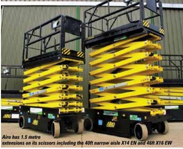
EW has very similar specifications and features but offers a 16 metre working height, 250kg capacity and an overall width of 1.2 metres. Total weight is the same at 3,600kg.
