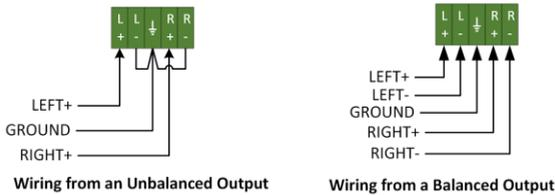
Note that the “LEFT-” and “RIGHT-” inputs are both linked to the ground connection when wiring from an unbalanced audio output. For a balanced audio input, wire all five connections from the balanced audio output as shown.
