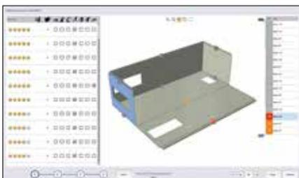
The best bending sequences are shown according to the highest the 5-star ranking.
