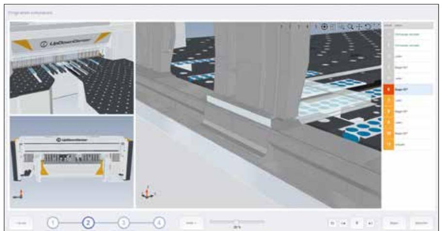
The 3D simulation shows the folding sequence and possible collisions. New products can already be evaluated during the design process.
