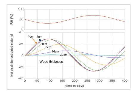
Figure 6. Strain in restrained wood (pine, radial) during an annual RH cycle with summer peak 70 % RH and winter trough 30 % RH, at 20 °C. for various thicknesses of wood. Thicker wood responds less, and its peak response is shifted more relative to the RH cycle. Calculated with 2000 time steps, 5 per day. Started with 0 stress at time 0. For simplicity, 1-year RH cycle set to 360 days
