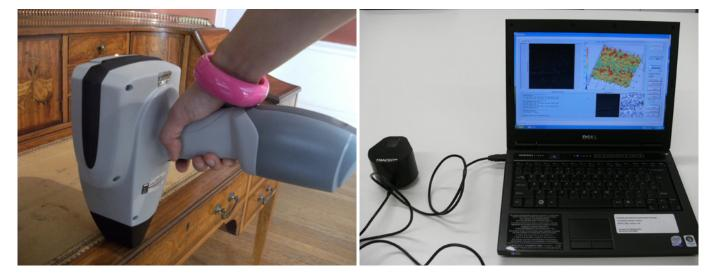
Figure 4. Near-infrared spectrum being recorded on the Carlton desk at Kenwood House
