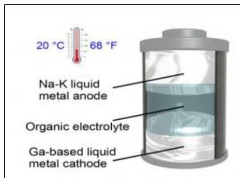
Schéma nové baterie. Kredit: University of Texas at Austin.
