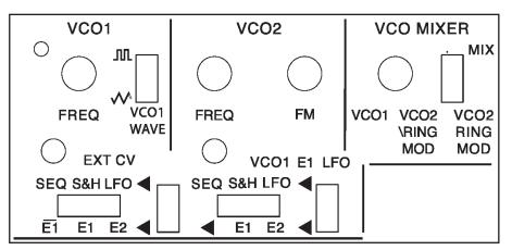
Each voo has two selectors, 2 and 3 way, it is possible to choose 6 different CV inputs
