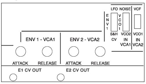
Generates an ATTACK ramp followed by a RELEASE ramp every pulse from: ENV1 instrument (Yellow LED) or ENV2 (Blue LED), ENV1 can be routed to VCO1, VCO2, VCA1 and CUT MOD, it has also negative output. ENV2 can be routed to VCO1. VCO2, VCA2 and RES MOD.
