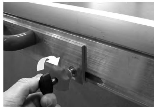
Figure 2: Screwing in the T-head bolt
