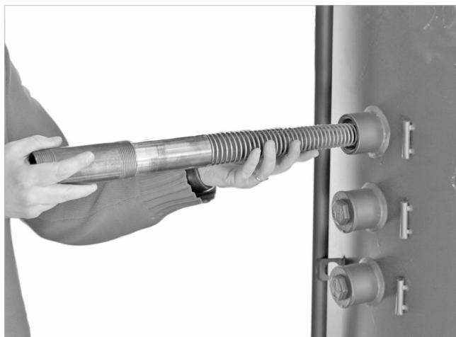
Fig. 3: Inserting and sealing the charging lance
