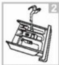
Clean the dispenser drawer and the softener cover under water
