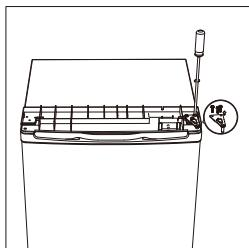
4. Unscrew bottom hinge. Then remove the adjustable feet from both side.
