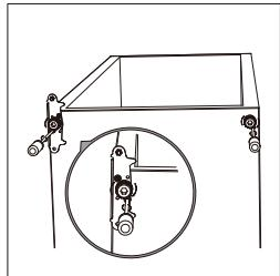
7. Place the door back on. Ensure the door is aligned horizontally and vertically, so that the seals are closed on all sides before finally tightening the top hinge.
