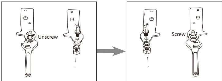
6. Refit the bracket fitting the bottom hinge pin. Replace both adjustable feet.
