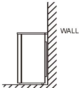
**⚠ Ensure that the appliance does not stand on the electrical supply cable.**
