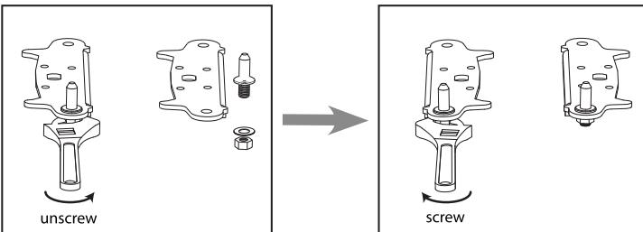
5. Refit the bracket fitting the bottom hinge pin. Replace both adjustable feet. Transfer the lower door to the property position.
