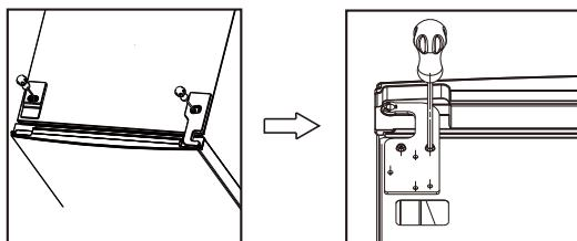
2. Unscrew from the middle hinge by cross screwdriver, then take off the lower door.
