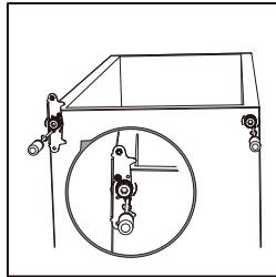
6. Make the middle hinge reverse the direction 180°C, then transfer it to the left property position.
