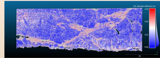
Figure 5. Cloud to cloud accuracy, when compared with the reference laser scan, was high on bare rock face, but low in vegetated areas and those with large depth discontinuities
