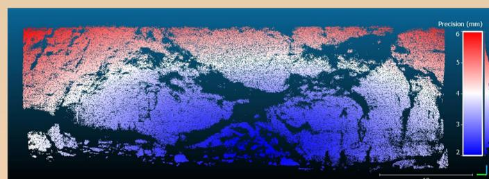
Figure 4. Points are most precise where image overlap is high, and distance to the target is lowest. Areas containing vegetation were generally not included within the sparse cloud.
