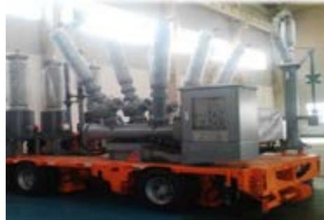
**Hybrid gas insulated switchgear**
