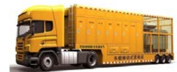
Photo of transformer trailer of 40.5 kV trailer substation
