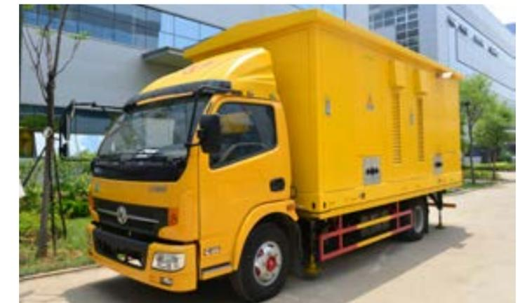
Photo of 12kV/0.4kV Trailer mobile substation
