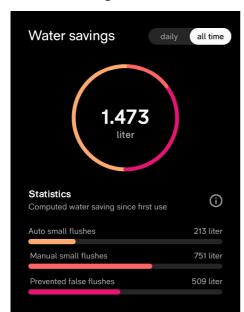
Water savings gives an overview of the amount of water saved. The metrics can be shown over the total lifespan of the product or as a daily average, by tapping the toggle switch in the top right corner.
