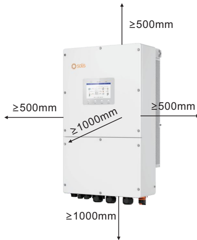
Figure 3.5 Inverter Mounting Clearances
