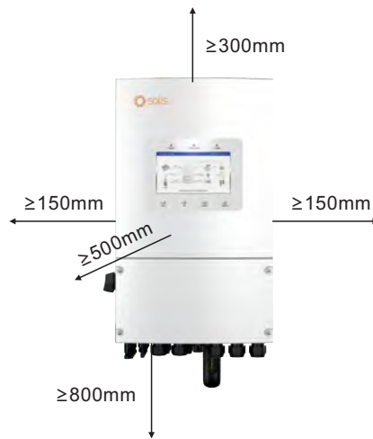
Figure 3.5 Inverter Mounting Clearances
