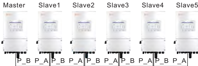
Figure 3.24 Parallel Terminal Connection
