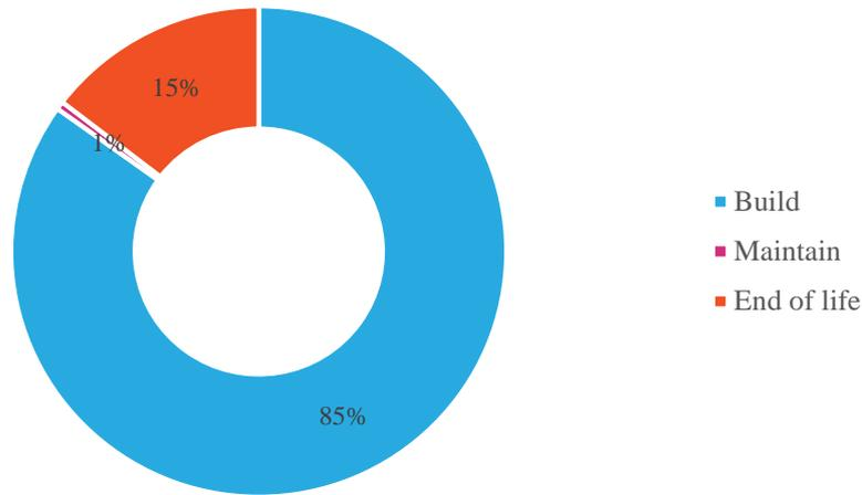
Figure 5 CO<sub>2</sub> MKI-value per life phase of the bridge
