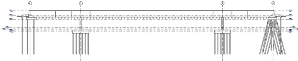
Figure 8 Section of the steel design for the Zuidhorn railbridge. ©ProRail.
