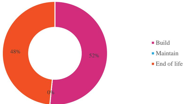
Figure 9 CO<sub>2</sub> MKI-value per life phase of the bridge
