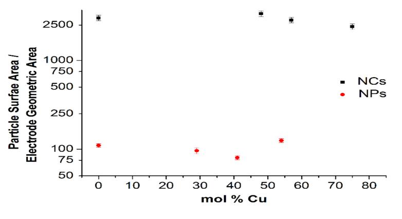
Pb UPD experiments of nanoclusters (black) and nanoparticles (red) in an Ar-sparged solution containing 100 mM HClO<sub>4</sub>, 1 mM Pb(ClO<sub>4</sub>)<sub>2</sub>, and 20 mM KCl at a scan rate of 10 mV/s
