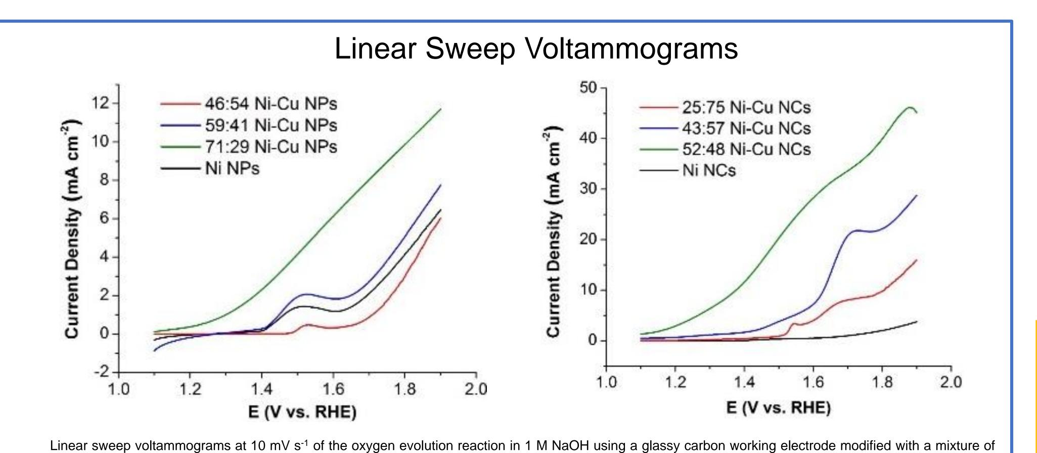
Ni-Cu bimetallic nanoparticles (NPs) or nanoclusters (NCs), Vulcan XC-72, and PVDF. Current densities are reported against the geometric electrode area.
