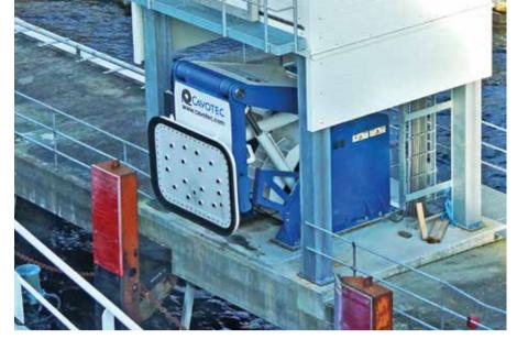
The vacuum system on shore- both ships are anchored rapidly and safely to harbor quays by using a vacuum system instead of conventional anchors.
