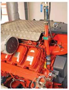
Diesel engine, used in case of batteries running out due to long trip or rough weather.
