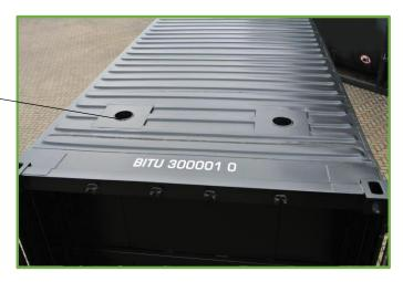
Manlid/manhole used or loading the bitumen
