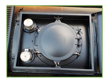
Walkways, cladding (50mm thick) and frame are refurbished to an acceptable level for certification and cosmetic purpose as well. All decals are replaced and the tank is painted in a black colour.
