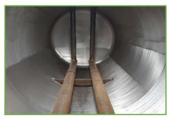
The flame tube system is certified by Germanischer Lloyds and compatible with IMO/ADR/RID/USDOT regulations. The IMO2 / T3 / L2.65BN codes will be applicable.
