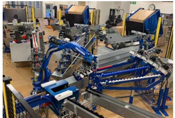
Automated assembly of racing lane line
