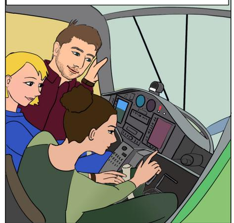
A GLASS COCKPIT, WITH A PRIMARY FLIGHT DISPLAY AND A MULTI-FUNCTION FLIGHT DISPLAY
