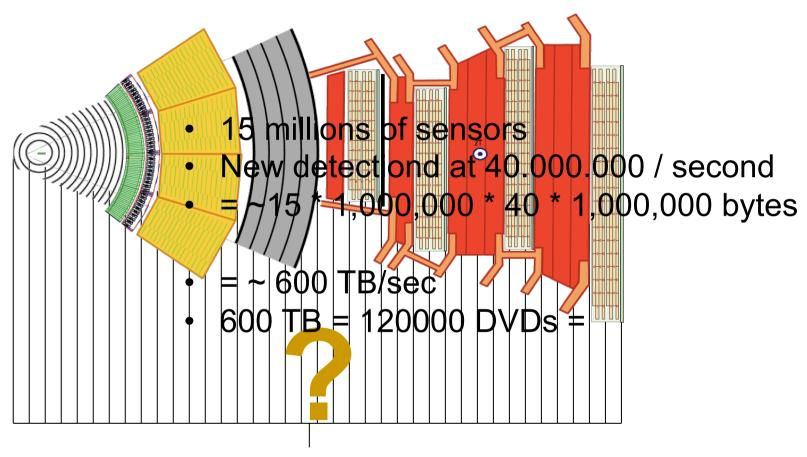
A detector is like a 3-D camera taking a photo 40 millions times per second, without the possibility of data compression
