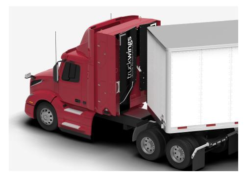
Panels fully retract at low speeds to maintain turning clearance with zero driver intervention required
