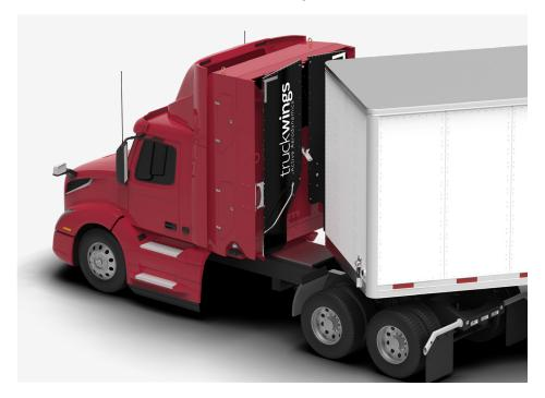
Panels fully retract at low speeds to maintain turning clearance with zero driver intervention required
