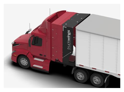
Patented folding panels deploy automatically to close the gap and streamline the tractor-trailer at highway speeds
