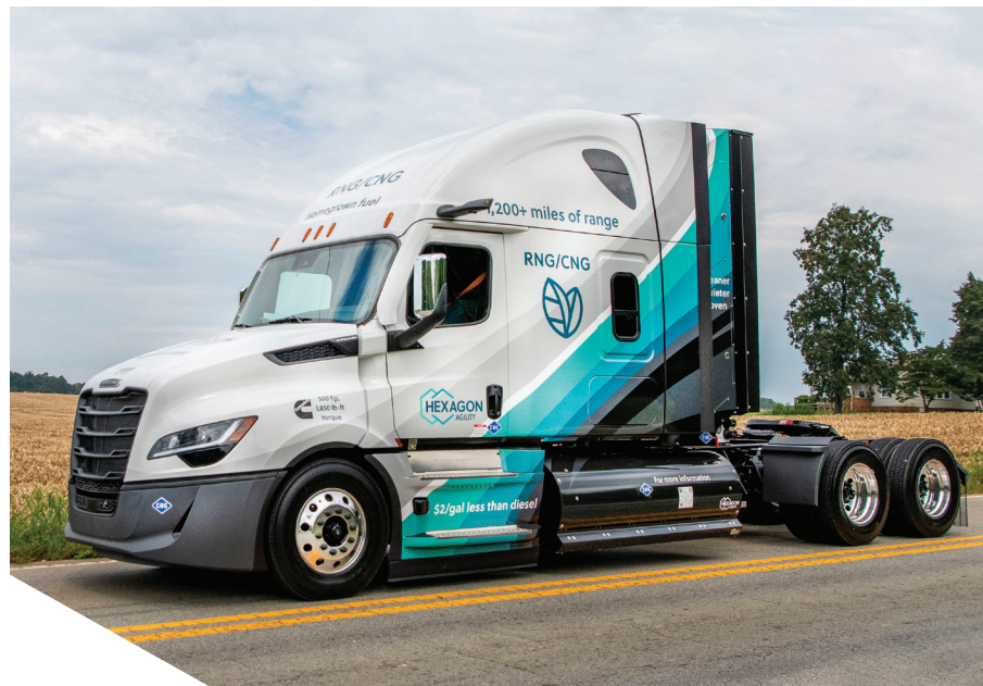
CNG 2026 Freightliner Cascadia 126 SLP, X15N, ProCab 175, dual ProRail 45
