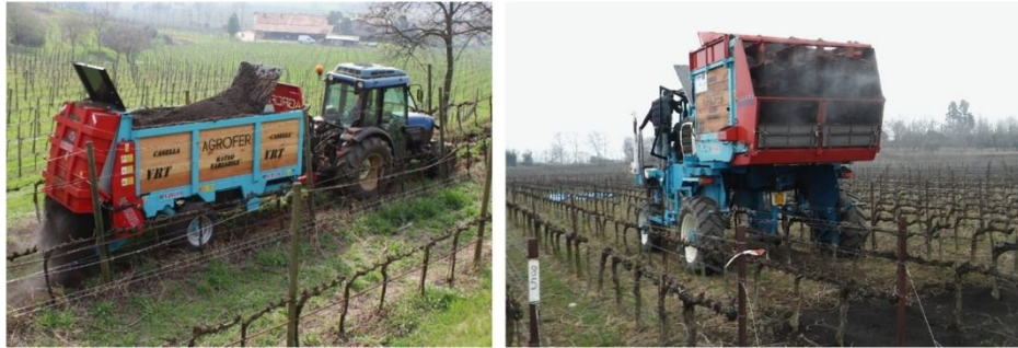
Figure 2 Two of the spreader prototypes manufactured for the Vitisom project: the towed self-levelling (left) and the straddle self-propelled (right) models
