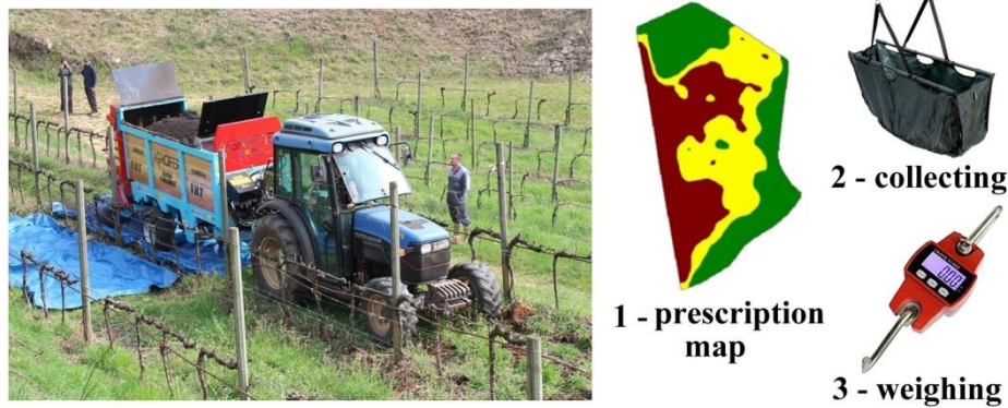
Figure 4 The amount of matrix distributed by the machine in each inter-row surveyed, and collected on the plastic sheets of known surface (left), was later weighed by using a digital dynamometer and compared with the expected figure resulting from the prescription map (right)
