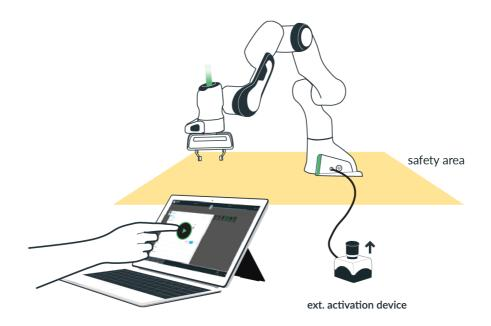
To test a program, before automatic execution is launched, the user needs to change the **External Activation Device** to the "**up**" position. Afterwards the user steps back and remains outside the safety area to run the test. Please make sure that the External Activation Device is positioned outside of the safety area and in immediate reach of the user.
