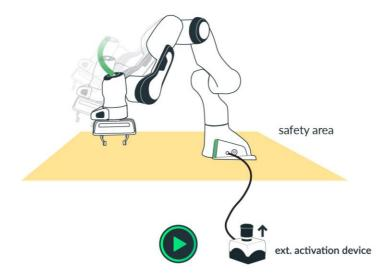
Once the user has verified that the robotic task is ready to be executed automatically, the **External Activation Device** remains in the "**up**" position (see figure above). By doing so, the user acknowledges that no one is or can enter the safety area around Panda during automatic execution. Please make sure that the External Activation Device is positioned outside of the safety area and in immediate reach of the user.
