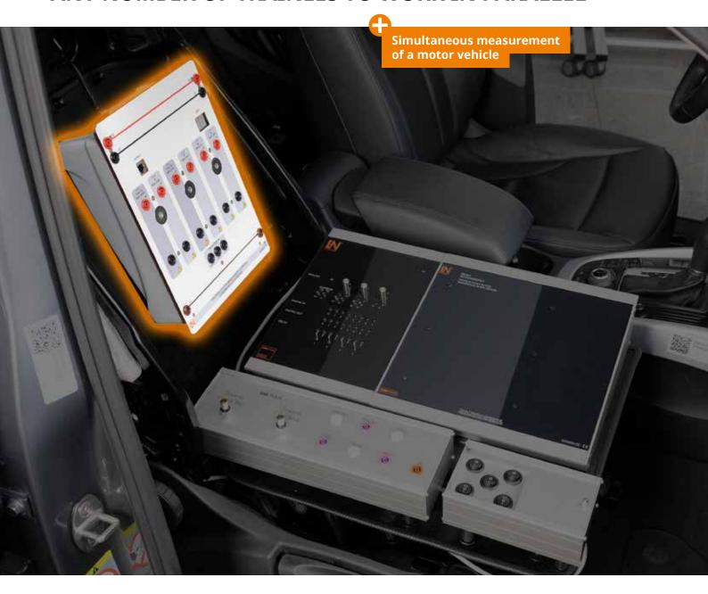
The measurement expansion package permits multiple trainees to conduct measurements and perform diagnostics at the same time on just one vehicle thanks to the inclusion of the student measurement stations.
