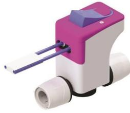
The Waterlock Valve is a secondary stopcock which isolates the mains water supply into the test property. It is controlled by the Valve Controller and will be professionally installed near your existing stopcock. The valve requires no power – it is driven by water pressure alone.
