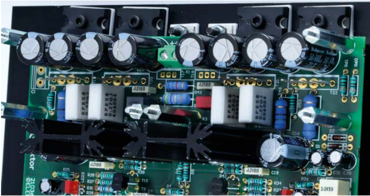
Figure 28. View of the PCB and the output stage transistors provisionally secured to the heatsink.
