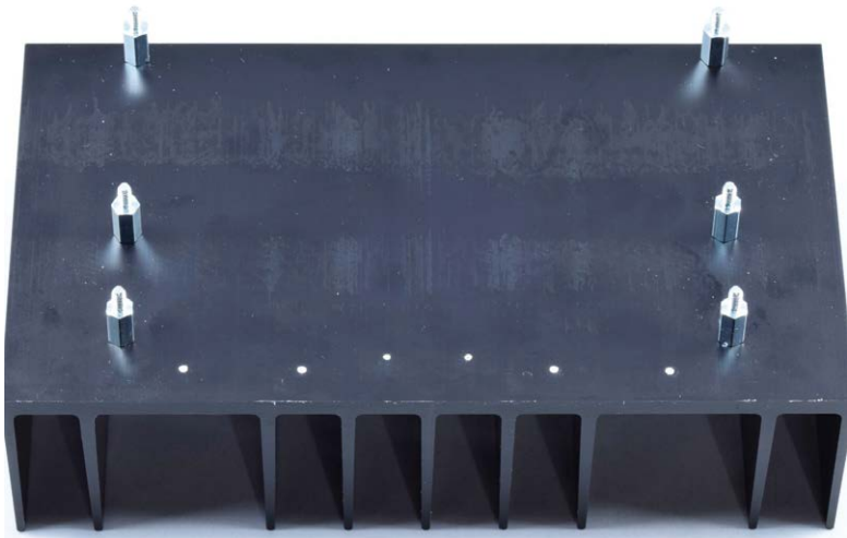
Figure 15. Marked-out positions for the six holes to be drilled (prototype).
