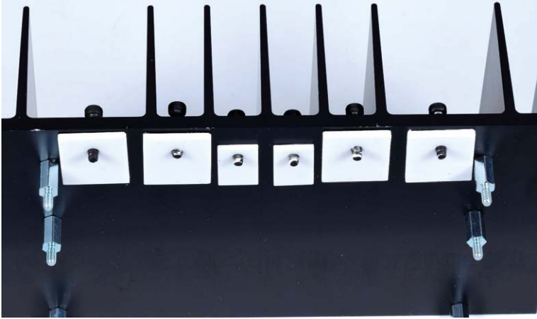
Figure 30. Slide the ceramic washers (pads) over the screw threads before positioning the PCB with the transistors.
