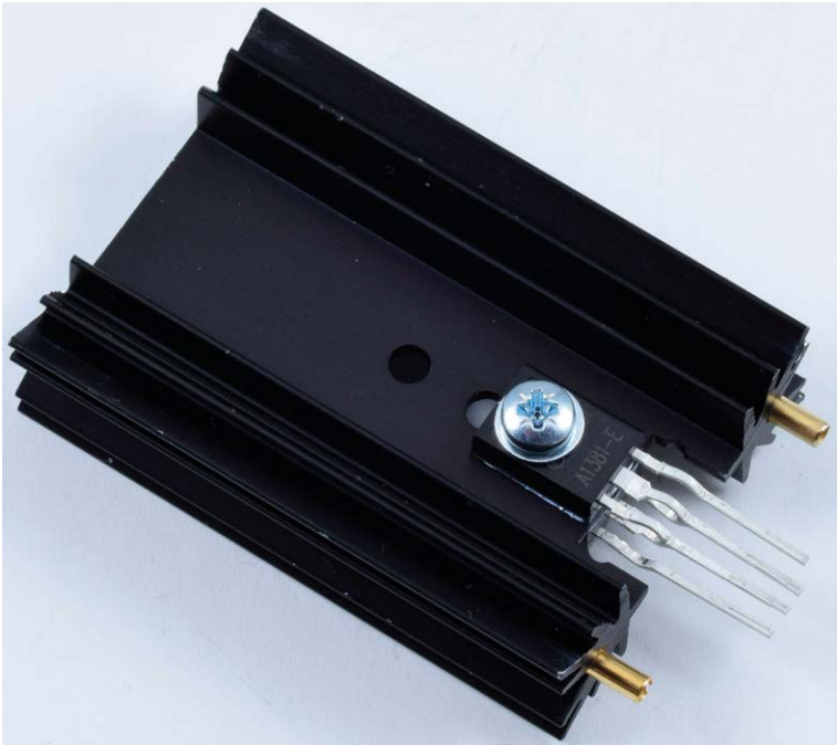
Figure 26. Two transistors mounted at each side of the small heatsink.
