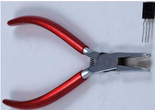
Figure 25. Special pliers and an example of the "thermal relief" bend in the leads needed for T13...T16.
