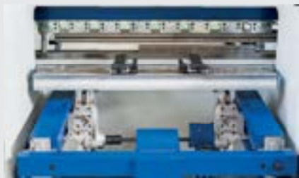
Standard X + R Axis Back Gauge
