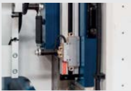
Standard GVI Optic Linear Scales
