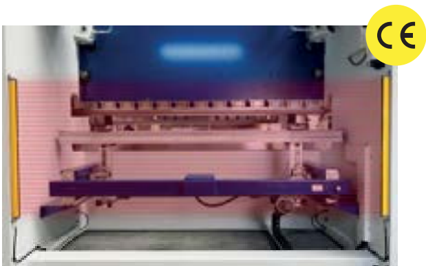
Rear Safety Light Curtain
