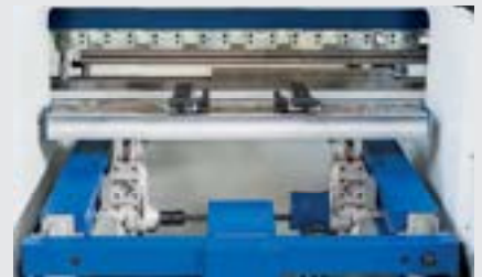
Standard X + R Axis Back Gauge
