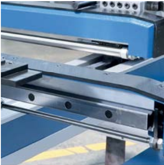
Pneumatic Rear Sheet Metal Support Arms
